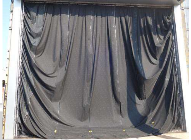
A2. EPDM rubber covered the whole surface area of Mock up specimen
